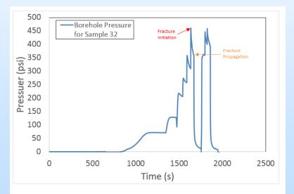
Figure 3.4: Borehole Pressure Profile of Sample #32.
