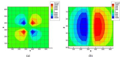
Figure 4.2.6. Shear  $\underline{xy}$ -stress cross sections for  $\underline{xy}$ -plane, K=5 (a) and  $\underline{xz}$ -plane, J=9 (b) after three years of injection.
