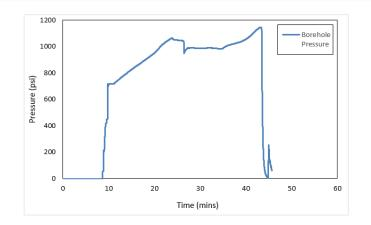
Figure 3.28: Borehole pressure during CO<sub>2</sub> injection.
